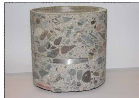
Core sample showing consolidation above and below plate
