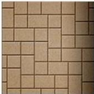
Modified Herringbone 60% 6 x 9 and 40% 6 x 6
